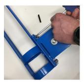
3) Attach the winch (D) to the long sleeve (H) using the 4 button head screws, the holes are threaded so no bolts are required (E).
