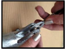
Put thimble inside net cable loop (C). Put cable between tag & insert bolt & tighten (A+B+C).
